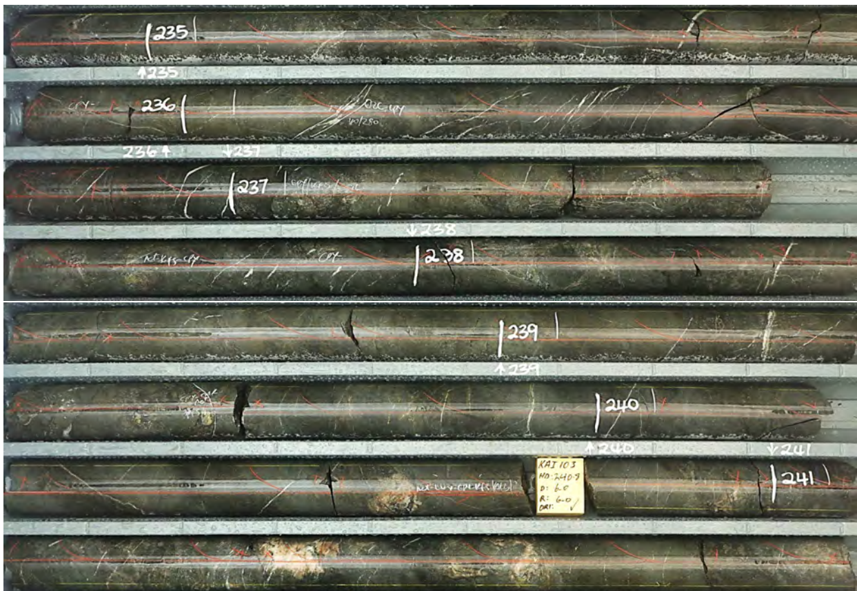
KAI103 (235m – 242m) – Monzonitic intrusive-hydrothermal breccia with calcite-actinolite-chalcopyrite. Photographed interval graded 7m at 1.50g/t AuEq* (0.74% Cu, 0.49g/t Au) from 235m.
